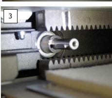
The frames are now free to move. Manually move the frame over the entire course to ensure that they slide properly.
